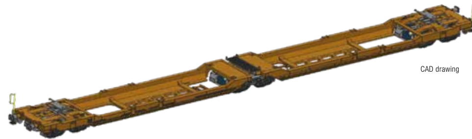
■ Trestle in a high position for semi-trailers and a low position for loading containers
