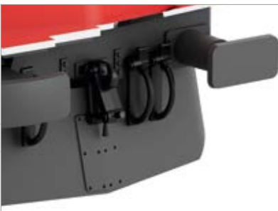
■ Buffer beam can be fully retrofitted
