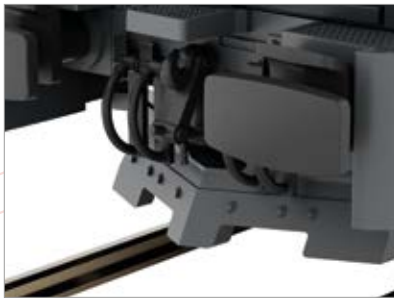
■ Buffer beam completely covered
